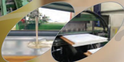
This is our panel forming plant at Peterlee. All 103 metres of it. The only one in the UK and capable of forming panel at 6 metres a minute.
